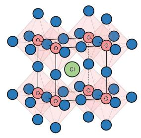
Fig. 1  $Na_3OCl$  anti-perovskite structure highlighting the cornersharing  $ONa_6$  octahedra available for Na-ion migration. Na ions are shown in blue.
