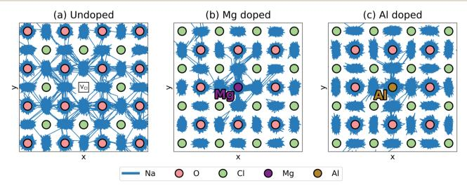
Fig. 5 Trajectory lines for Na-ion migration with a 0.27% Na-vacancy concentration (a) undoped system, (b) Mg-doped system and (c) Al-doped system. The first 2 ns and a  $3 \times 3 \times 3$  fraction of the supercell at 900 K are shown. O, Cl, Mg and Al ions are brought to the foreground for clarity, but it is important to note that not all of the ions occupy the same plane.
