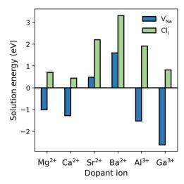
Fig. 2 Dopant solution energies for M<sup>2+</sup> and M<sup>3+</sup> doping in Na<sub>3</sub>OCl based on eqn (7)-(10). Metal chlorides were used as doping agents in the reactions.
