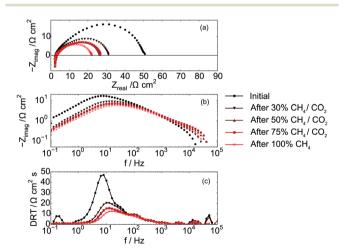
Fig. 5 Impedance data for a cell with a Ni–Co–CGO anode measured in 3%  $\rm H_2O/H_2$   $\rm H_2$  at 750 °C (reference conditions) after operation in various  $\rm CH_4/CO_2$  atmospheres at 750 °C for 15 minutes each. (a) the Nyquist representation (b) in the Bode representation and (c) distribution of relaxation times.
