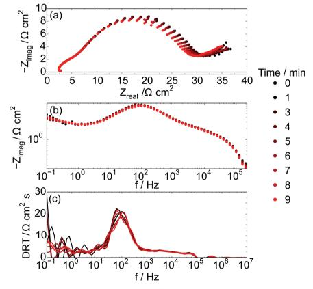
Fig. 7 Impedance spectra recorded during the strongest polarization (85%  $I_{max}/5.5$  mA) of the Ni–Co–CGO cell in 100% CH<sub>4</sub> at 750 °C; (a) plotted as Nyquist plots and (b) plotted as Bode plots, (c) DRT representation.
