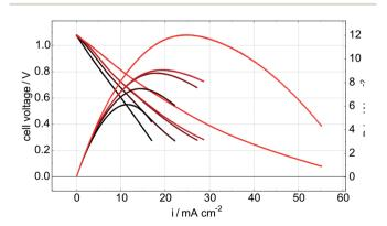
Fig. 4 LSV curves for a cell with a Ni–Co–CGO anode measured in 3%  $H_2O/H_2$  at 750 °C (reference conditions) after operation in various  $CH_4/CO_2$  atmospheres at 750 °C for 15 minutes each. The LSV curves (left axis) are plotted together with the calculated power curves (right axis).
