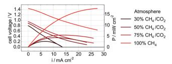
Fig. 6 LSV and power density curves of a cell with a Ni-Co-CGO anode measured in 30% CH<sub>4</sub>/CO<sub>2</sub>, 50% CH<sub>4</sub>/CO<sub>2</sub>, 75% CH<sub>4</sub>/CO<sub>2</sub>, and 100% CH<sub>4</sub> at 750 °C.
