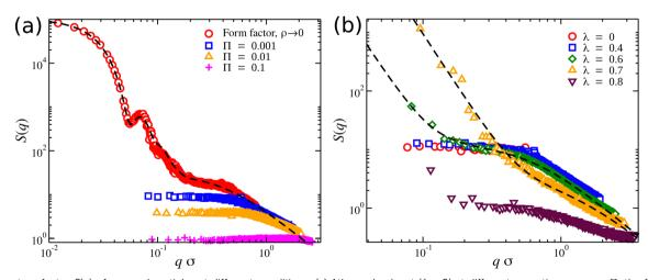
Fig. 9 Structure factor S(q) of nanogel particles at different conditions. (a) Athermal solvent ( $\lambda = 0$ ) at different osmotic pressures  $\Pi$ ; the form factor (dashed line) of an isolated nanogel particle is also presented along with a fit to the "extended fuzzy sphere" model.<sup>20</sup> (b) Different solvent qualities at osmotic pressure  $\Pi$  = 0.0001; the dashed lines are fits with eqn (10)
