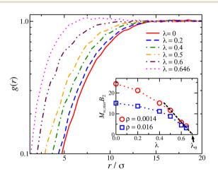
Fig. 7 Pair correlation function, g(r), for center of mass star polymer (f = 4 arms and M = 25 arm length) solution at a segmental density  $\rho\sigma^3 \approx 0.016$ . Inset: Second virial of star polymer solutions as a function of  $\lambda$ ; results at different polymer concentrations are also presented. The dashed line is an extrapolation to identify the  $\theta$ -point at  $B_2 = 0$ .
