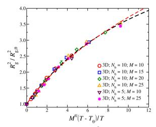
Fig. 5 Average square radius of gyration,  $R_q^2$ , of isolated compact nanogel particles normalized by  $R_q^2$  at  $\theta$ -point, as a function of the reduced temperature,  $\tau = (T - T_{\theta})/T$  and chain length, M, scaled with an exponent  $\varphi$ . The dashed line is a fit of eqn (5) with  $\nu$  = 1/2 (black line) and  $\nu$  = 0.588 (red line). The uncertainty estimates correspond to two standard deviations.
