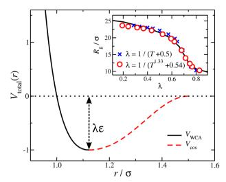
Fig. 1 The non-bonded, bead-bead interaction potential V(r) with  $\lambda = 1$ , showing the contributions from  $V_{WCA}(r) + V_{SW}(r)$  (black) and  $V_{cos}(r)$  (red). Inset: Average radius of gyration of a nanogel particle  $via \lambda$  variation (black line) and temperature T variation (symbols). Two relations between  $\lambda$  and Tare presented.
