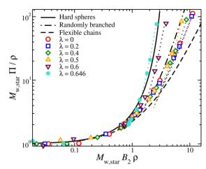
Fig. 8 Compressibility factor,  $M_{w,star}\Pi/\rho$ , for compact nanogel particles (dotted lines) and star polymer solutions (symbols), as a function of  $B_2 M_{\text{\tiny MM}} \rho$ for different values of solvent quality parameter,  $\lambda$ . The cases of hard spheres based on the Carnahan-Starling, 71 flexible chains, 72 and randomly branched structures<sup>56</sup> are also presented.
