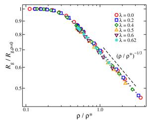
Fig. 6 Average radius of gyration normalized by its value of infinite dilution,  $R_{\rm g}/R_{{\rm g},\rho=0}$  as a function of the reduced segmental density,  $\rho/\rho^{\star}$ , where  $ho^*=rac{4\pi}{3}R_{\mathrm{g},
