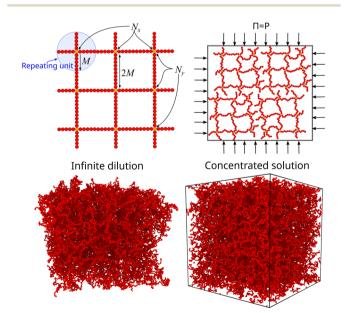
Fig. 2 Schematic of the molecular architecture of the nanogel particle. Typical screenshots of a equilibrated molecular configuration of compact nanogel particle at infinite dilution (the simulation box is so large that is not visible) and fixed osmotic pressure conditions, where the nanogel particles fill the simulation box and interacting through periodic boundaries.
