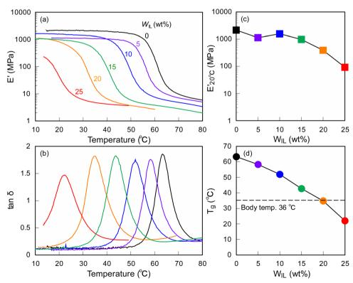
Fig. 2 Temperature dependence of (a) storage modulus (E') and (b) loss tangent (tan  $\delta$ ) for ionic SMP gels with different  $W_{IL}$ . Dependence of (c) storage modulus at 20 °C  $(E'_{20\,^{\circ}\mathrm{C}})$  and (d)  $T_{\mathrm{g}}$  of ionic SMP gels on  $W_{\mathrm{IL}}$ .
