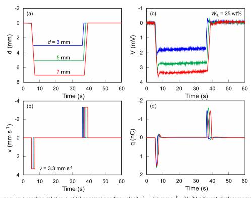
Fig. 7 Relation between input mechanical stimuli of (a) constant bending velocity ( $v = 3.3 \text{ mm s}^{-1}$ ) with (b) different displacements (d = 3, 5, 7 mm) and output electric signals of (c) voltage (V) and (d) electric charge (q) of ionic SMP gel sensor ( $W_{IL} = 25 \text{ wt}\%$ ).
