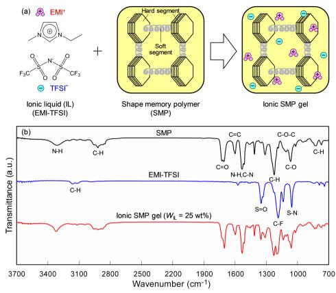
Fig. 1 (a) Schematic illustration of ionic shape memory polymer (SMP) gel composed of ionic liquids (EMI-TFSI) and SMPs. (b) FT-IR spectra of SMPs, EMI-TFSI, and ionic SMP gels ( $W_{\rm IL}$  = 25 wt%).
