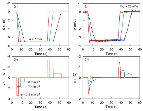
Fig. 6 Relation between input mechanical stimuli of (a) constant bending displacement (d = 7 mm) with (b) different velocities (v = 0.8, 1.7, and3.3 mm s<sup>-1</sup>) and output electric signals of (c) voltage (V) and (d) electric charge (q) of ionic SMP gel sensor ( $W_{\rm IL} = 25$  wt%).
