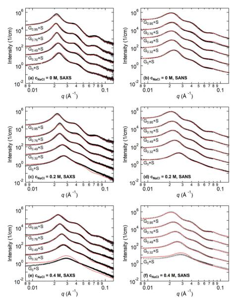
Fig. 3 SAXS and SANS profiles for 8 wt%  $G_x$  + S hydrogels at  $c_{NaCl}$  = 0, 0.2, and 0.4 M, where x denotes the molar percentage of the guanidinium moiety over total cations in the end-block of the triblock copolymer. Solid curves represent the best fit to the fitting model. Data and curves are vertically shifted for clarity.
