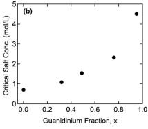
Fig. 6 Effects of the guanidinium fraction, x, on (a) the interfacial tension at the zero-salt limit,  $\gamma_{\text{core},0}$ , and (b) the critical salt concentration,  $c^*$ , of the complex coacervates. The inset in (a) compares  $\gamma_{\text{core},0}$  with the polymer fraction in the coacervate core at the zero-salt limit,  $f_{\text{core},\text{pol},0}$ .
