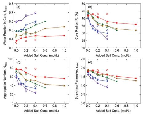
Fig. 4 SAXS (closed symbols) and SANS (open symbols) fit results from  $G_0 + S$  (purple/hexagons),  $G_{0.32} + S$  (blue/diamonds),  $G_{0.49} + S$  (green/triangles),  $G_{0.76} + S$  (brown/squares), and  $G_{0.95} + S$  (red/circles) hydrogels as functions of the added salt concentration. (a) Water fraction in the coacervate core, (b) core radius, (c) aggregation number, and (d) dimensionless parameter of the PEO chain stretching.
