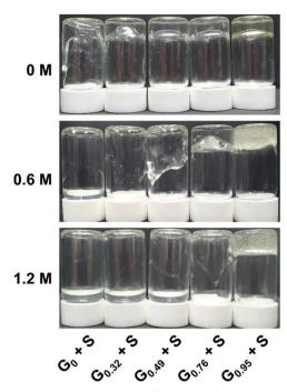
Fig. 2 Representative photographs of 8 wt%  $G_x$  + S hydrogels at  $c_{NaCl}$  = 0, 0.6 and 1.2 M. Vials were inverted for 20 s before the snapshot was taken.
