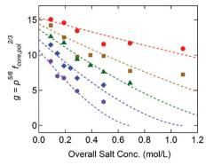
Fig. 5 Dimensionless parameter for the interfacial tension,  $g = p^{5/6} f_{\text{core nol}}^{2/3}$ as a function of the overall salt concentration for  $G_0 + S$  (purple/hexagons),  $G_{0.32}$  + S (blue/diamonds),  $G_{0.49}$  + S (green/triangles),  $G_{0.76}$  + S (brown/ squares), and  $G_{0.95}$  + S (red/circles). The dashed lines are the best fits to the model function of  $g = g_0(1 - c_s/c^*)^{3/2}$ .
