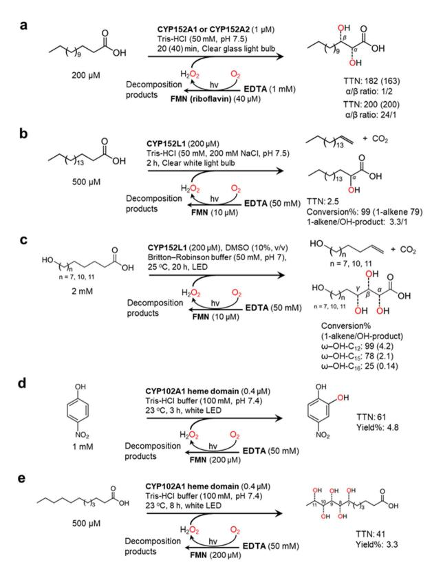
Fig. 5 Photochemically driving P450 peroxygenases using FMN as a photocatalyst and EDTA as an electron donor. Hydroxylation of fatty acids<sup>101–103</sup> (a and b) and ω-hydroxylated fatty acids<sup>104</sup> (c) is catalyzed by CYP152 peroxygenases. CYP102A1 heme domain also shows peroxygenase activity towards 4-nitrophenol (d) and lauric acid (e).<sup>12</sup>
