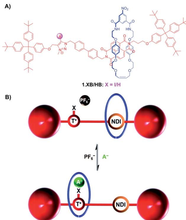
Fig. 6 (A) Chemical structure of bistable (iodo)triazolium-NDI [2] rotaxanes **1.XB/HB**. (B) Schematic depiction of anion recognition-induced shuttling of the macrocycle from the NDI to the triazolium, resulting in a naked-eye colour change from orange to colourless due to disruption of the donor-acceptor charge-transfer interactions between the hydroquinone-containing macrocycle and the NDI station. Reproduced from ref. 90 with permission from the Royal Society of Chemistry.
