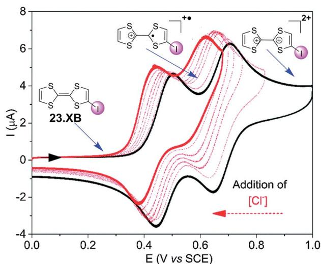
Fig. 24 Chemical structure of iodo-TTF **23.XB** and its corresponding CV in DMF in the absence (black) and presence (red) of increasing concentrations of  $\text{Cl}^-$ . Depicted are also the different redox states at different potentials (structures and blue arrows). Adapted from ref. 138 with permission from the PCCP Owner Societies.
