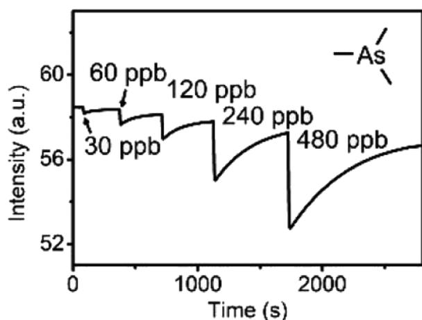
Fig. 19 Fluorescence emission intensity of bundled nanoribbons of **16.ChB** upon exposure to increasing concentration of trimethylarsine gas. Reproduced with permission from ref. 131 copyright 2021 American Chemical Society.
