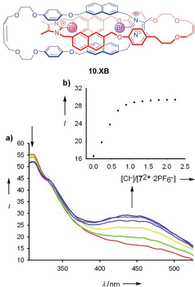
Fig. 13 All-XB bromo-imidazolium-naphthalene catenane **10.XB** for fluorescent halide sensing. (a) Emission spectra of 10 μM **10.XB** upon addition of Cl<sup>-</sup> in ACN. (b) The corresponding response isotherm at 445 nm. Reproduced with permission from ref. 122 copyright 2011 Wiley.
