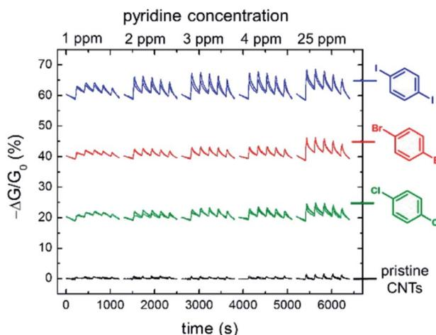
Fig. 37 Conductance response of chemiresistive gas sensors containing different dihaloaryl XB selectors in the repeating presence of increasing concentrations of pyridine in  $N_2$  carrier gas. For clarity the relative conductance responses are offset by 20%. Reproduced with permission from ref. 171 copyright 2016 American Chemical Society.
