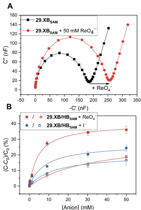
Fig. 34 (A) Capacitive Nyquist plots of  $29.XB_{SAM}$  in the absence and presence of 50 mM  $\text{ReO}_4^-$  showing an increased capacitance in the presence of bound anion. (B) Relative capacitive sensor response of  $29.XB_{SAM}$  (filled symbols) and  $29.HB_{SAM}$  (empty symbols) in response to  $\text{ReO}_4^-$  (red) and  $\text{I}^-$  (blue). Reproduced from ref. 162 with permission of the Royal Society of Chemistry.
