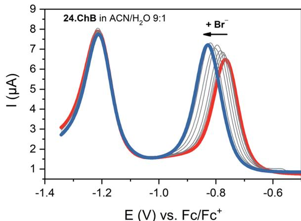
Fig. 27 SWVs of telluroviologen ChB sensor **24.ChB** in ACN/H<sub>2</sub>O 9 : 1 upon addition of up to 50 mM Br<sup>-</sup>. Only the first reductive couple is responsive, indicative of complete ChB deactivation upon mono-reduction. Reproduced with permission from ref. 62 copyright 2022 American Chemical Society.
