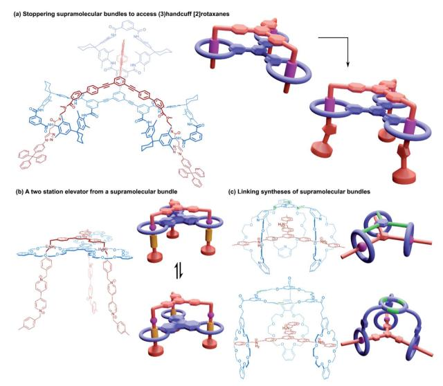
Fig. 11 (3)Handcuff [2]rotaxanes. (a) The stoppering of a supramolecular bundle made from a tris(tetralactam) host via azide—alkyne cycloadditions to give a (3)handcuff [2]rotaxane; (b) a two station molecular elevator with a platform that moves between viologen and dibenzy-lammonium stations; (c) linking synthesis of supramolecular bundles using olefin metathesis and imine formation.
