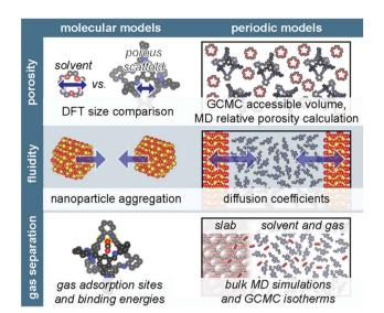
Fig. 4 Common molecular (left panel) and periodic (right panel) models and methods are briefly outlined for three porous liquid properties; porosity (top), fluidity (middle), and gas adsorption (bottom). Hydrogens omitted for clarity.
