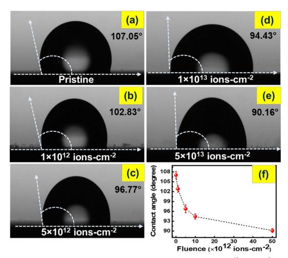
Fig. 14 Contact angles (CA) of (a) pristine film, and absorber films developed at different fluences of (b)  $1 \times 10^{12}$  ions per cm<sup>2</sup>, (c)  $5 \times 10^{12}$  ions per cm<sup>2</sup>, (d)  $1 \times 10^{13}$  ions per cm<sup>2</sup>, and (e)  $5 \times 10^{13}$  ions per cm<sup>2</sup>. (f) Variation of CA with ion fluence. [Reproduced/adapted from Maity et al., 159 J. Appl. Phys., 2021, 129, 045301, with the permission from AIP Publishing.]
