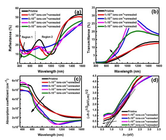
Fig. 17 (a) Reflectance, and (b) transmittance spectra of pristine sample and post-annealed (at 300 °C) samples after ion irradiation at different fluences. (c) Absorption coefficient and (d) plot of  $(\alpha h v)^{1/2} vs$ . photon energy (h v) for pristine sample and post annealed (at 300 °C) samples after ion irradiation at different fluences. [Reproduced/adapted from Maity et~al.,  $^{162}$  CrystEngComm., 2020, **22**, 666, with permission from The Royal Society of Chemistry.]
