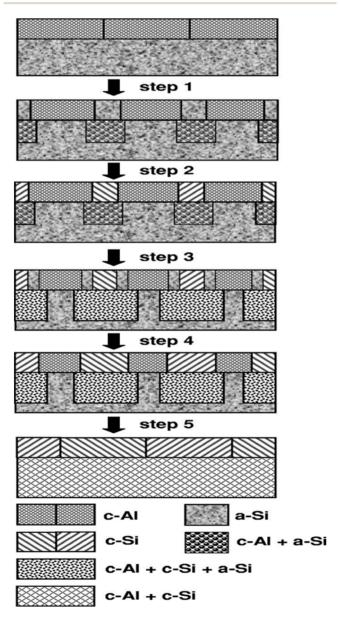
Fig. 1 A schematic presentation of the mechanism of the Al induced layer exchange process. [Reproduced/adapted from Wang et al., 16 J. Appl. Phys., 2007, 102, 113523, with the permission from AIP Publishing.]
