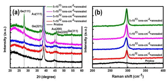
Fig. 12 (a) XRD pattern and (b) Raman spectra of pristine sample and samples post-annealed (after ion irradiation at different fluences) at 300 °C. The XRD and Raman results clearly show the crystallization of Ge due to thermal annealing treatment after ion irradiation. [Reproduced/adapted from Maity et al., 162 CrystEngComm, 2020, 22, 666, with permission from The Royal Society of Chemistry.]
