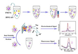
Fig. 5 Schematic diagram of fluorescence and electrochemical dualmode immunoassay platform for detection of avian influenza virus. Reproduced from ref. 39 with permission from American Chemical Society.
