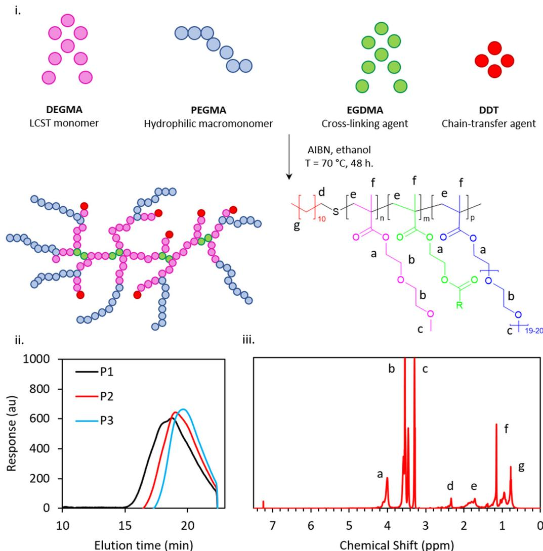
Fig. 1 Free radical polymerisation of PDEGMA-PEGMA-EGDMA-DDT and theoretical structure of the branched copolymer surfactant (BCS) (i), exemplar GPC chromatogram of P1–3 (ii) and exemplar  $^1\text{H}$  NMR spectrum (iii).
