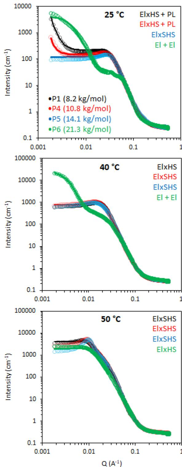
Fig. 8 SANS data (circles) with fits (lines) of 20 wt% BCS solutions in D<sub>2</sub>O with constructs of varying molecular weight and temperature. Legend inset with sample id and  $M_n$  determined by GPC. Models used to fit data are inserted top right. El is an ellipsoid form factor, HS and SHS are hard sphere and sticky hard sphere structure factors, respectively, whilst  $\times$  and  $+$  are mathematical operators. PL is a power law with a  $q^{-4}$  decay.
