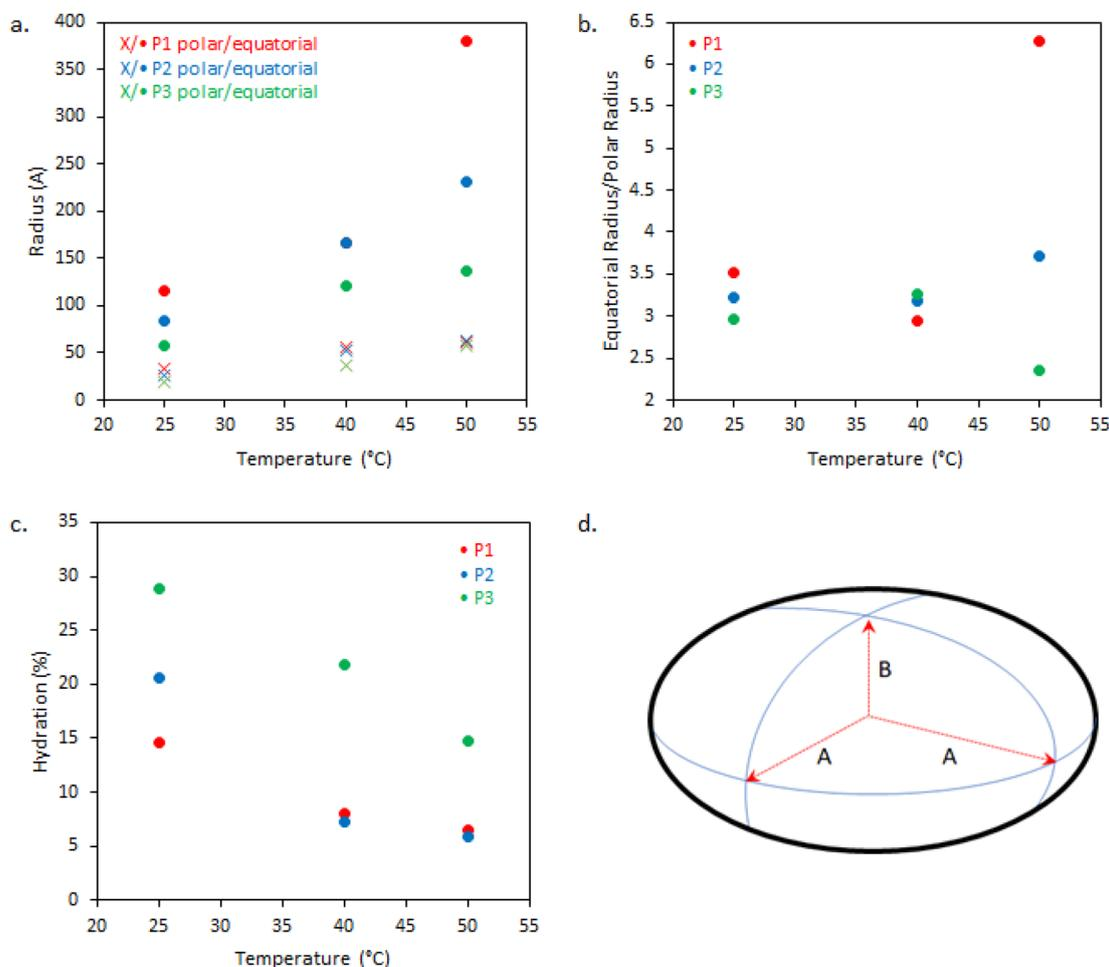
**Fig. 6** (a) Dimensions of BCS ellipsoidal aggregates with variation of cross-linking and temperature, derived from SANS fitting, (b) the ratio of equatorial to polar radii, and (c) degree of hydration of BCS particles estimated from SLD values obtained from the fits. (d) Shows the geometric structure of an ellipsoid where A and B are the equatorial and polar radii, respectively. When  $A > B$  the ellipsoid is oblate.
