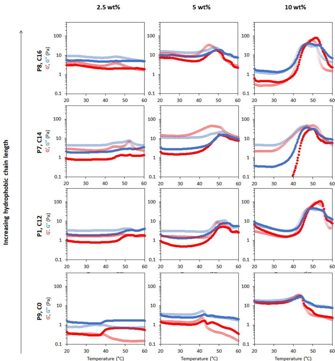
**Fig. 10** Effect of hydrophobic alkyl tail length on thermo-gelation activity of emulsions as determined by a rheology temperature ramp. P9 is synthesized with mercaptoethanol, P1 with dodecanethiol, P7 with tetradecanethiol and P8 with hexadecanethiol, leading to alkyl chain lengths of 0, 12, 14, and 16 C atoms, respectively.  $G'$  is shown in red and  $G''$  is shown in blue. Full rheograms showing the Y-axis region  $< 0.1$  Pa for P7 at 10 wt% are shown in Fig. S15.†
