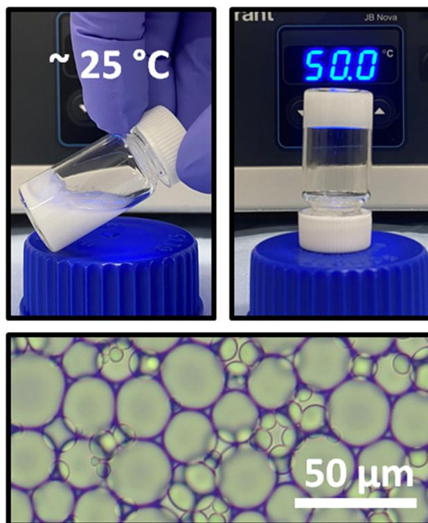
**Fig. 2** Dodecane-in-water emulsions stabilized by P1 BCS flow under the effect of gravity at room temperature but transition to a rigid gel state upon heating (top). Microscopy confirms the presence of oil droplets (bottom).
