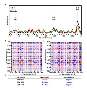
Fig. 5 (a) Raman spectra of 10 wt% PNIPAAm solutions in  $D_2O$  (black line), 0.5 M NaSCN (red line), and 1 M NaSCN (green line). 2DCOS (b) synchronous and (c) asynchronous spectra of PNIPAAm (10 wt%) with variation in the NaSCN concentration. (d) Peak descriptions for the 2DCOS results, where red is defined as a positive intensity, while blue is defined as a negative intensity.
