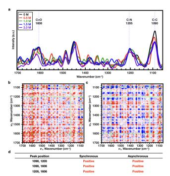
Fig. 7 (a) Raman spectra of 10 wt% of PiPOx in  $D_2O$  (black line), NaSCN 0.5 M (red line), NaSCN 1 M (green line), NaSCN 1.5 M (blue line), and NaSCN 2.0 M (purple line). 2DCOS (b) synchronous and (c) asynchronous spectra of PiPOx (10 wt%) depending on the NaSCN concentration. (d) Peak description of the 2DCOS result. Herein, red color is defined as a positive intensity, while blue color is defined as a negative one.
