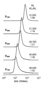
Fig. 2 SEC curves of PDMAAm macro-CTAs. Reaction conditions: see Table 1.
