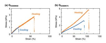
Fig. 8 Uniaxial tensile tests of (a) G<sub>D300N50</sub> and (b) G<sub>D300N75</sub> in heating and cooling states.
