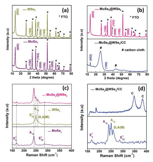
Fig. 3 XRD pattern (a) WSe<sub>2</sub> and MoSe<sub>2</sub> (b) MoSe<sub>2</sub>@WSe<sub>2</sub>/FTO and MoSe<sub>2</sub>@WSe<sub>2</sub>/CC. Raman spectra (c) WSe<sub>2</sub> and MoSe<sub>2</sub>@WSe<sub>2</sub>/FTO and MoSe<sub>2</sub>@WSe<sub>2</sub>/CC.
