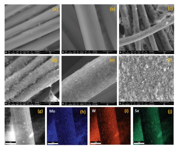
Fig. 5 (a) The schematic illustration of MoSe<sub>2</sub>@WSe<sub>2</sub> HS film deposition on carbon fiber cloth by EPD. SEM images of (b and c) bare carbon fibers and (d and e) MoSe<sub>2</sub>@WSe<sub>2</sub> HS-coated carbon fibers. (f-i) EDAX elemental mapping of MoSe<sub>2</sub>@WSe<sub>2</sub> HS on single CF.
