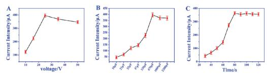
Fig. 6 (A) The voltage-current curve of capacitor with the same capacitance and different voltages; (B) the voltage-current curve of capacitor with the same voltages and different capacitance. (C) The charging time-current curve of 25 V and 470 µF capacitor.
