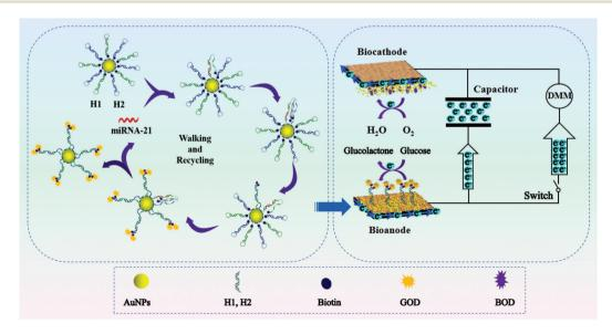
Scheme 1 Schematic illustration of enzyme-free 3-D DNA walking nanomachine based self-powered biosensing with triple signal amplification systems.
