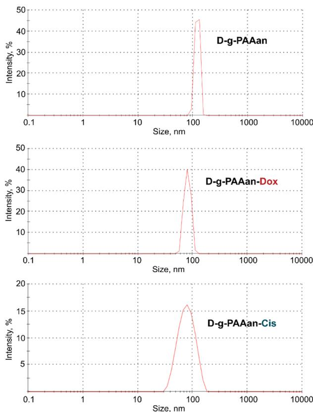
Fig. 1 Hydrodynamic size (diameter, nm) of free, Dox- and Cis-loaded D-g-PAAan particles; intensity in %: percentage of all scattered light intensity.
