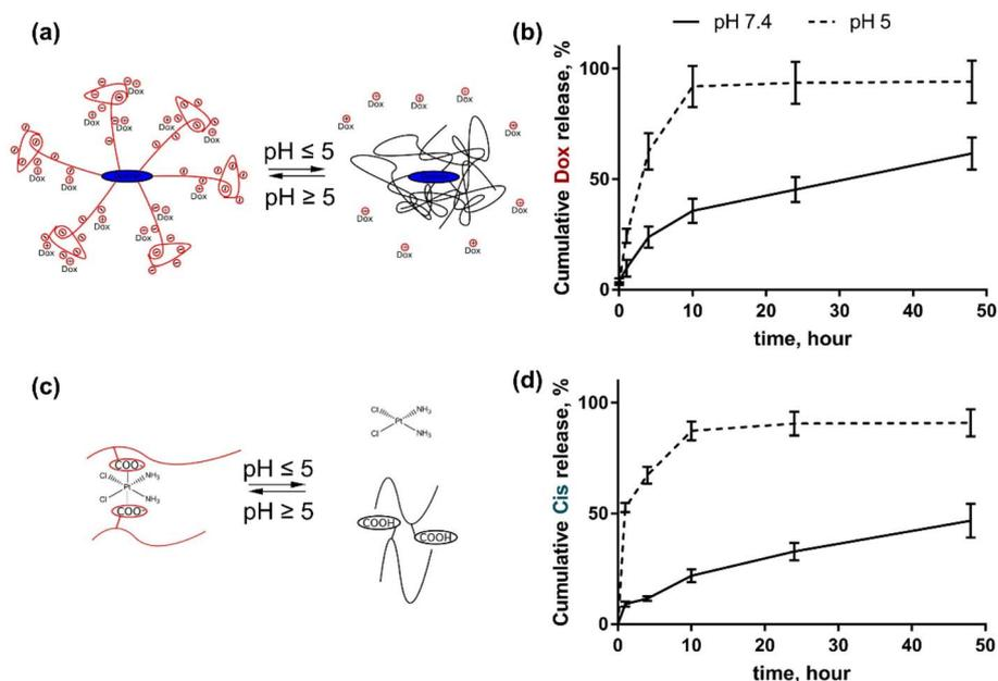
Fig. 2 Drug release from D-g-PAAan nanoparticles: schematic representation of Dox (a) and Cis (c) release; cumulative release of Dox (b) and Cis (d) during 48 h of incubation at pH 7.4 and 5.0.
