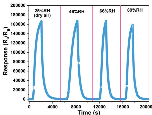
Fig. 10 The dynamic response curve of 0.5%Co-SnO<sub>2</sub> NPs under different humidity.
