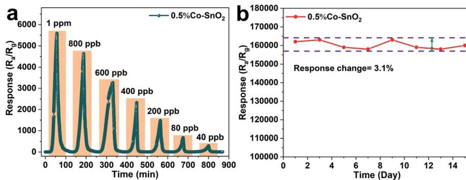
Fig. 7 (a) The response transients of 0.5%Co-SnO<sub>2</sub> NPs to ultra-low concentrations of formaldehyde, (b) long-term stability of 0.5%Co-SnO<sub>2</sub> NPs to 30 ppm formaldehyde at 90 °C.
