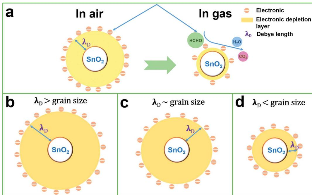
Fig. 11 (a) The cross-sectional view of the sensing mechanism of SnO<sub>2</sub> NPs in the presence of air and in formaldehyde; schematic of SnO<sub>2</sub> NPs grain size versus electron depletion layer thickness, (b) electronic depletion layer ( $\lambda_D$ ) > grain size, (c) electronic depletion layer ( $\lambda_D$ )  $\sim$  grain size, (d) electronic depletion layer ( $\lambda_D$ ) < grain size.
