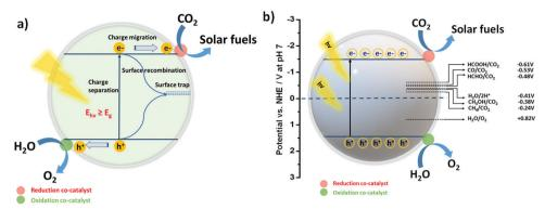
Fig. 1 (a) Schematic illustration of the elementary processes of photogenerated charges over the photocatalytic surface. (b) Schematic illustration of photocatalytic  $CO_2$  and  $H_2O$  conversion over a semiconducting photocatalyst for solar fuel production mediated by suitable redox co-catalysts.
