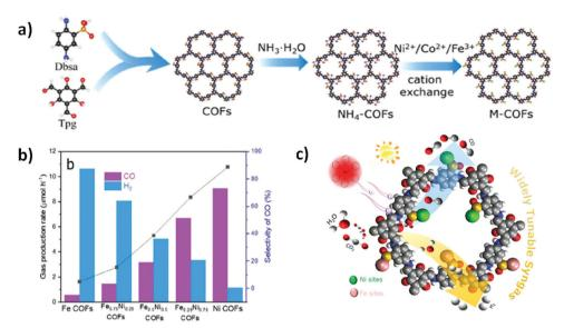
Fig. 10 (a) Synthesis of M-COFs with 2,4,6-triformylphloroglucinol (Tpg) and 2,5-diaminobenzenesulfonic acid (Dbsa) as the precursors. (b) The dependence of CO/H<sub>2</sub> ratios of metals in a series of Fe/Ni-COF samples in low-concentration CO<sub>2</sub>. (c) Schematic scheme for CO<sub>2</sub> reduction into CO and H<sub>2</sub>. Reproduced and modified with permission.  $^{41}$  Copyright 2020, Wiley-VCH.
