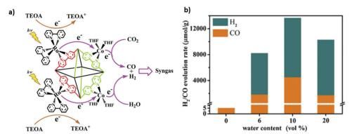
Fig. 8 (a) Proposed mechanism for photocatalytic syngas production with  $(Co/Ru)_n$ -UiO-67(bpydc) as the catalyst under the visible light irradiation. (b) Time profile of H<sub>2</sub> and CO evolution rate. Reproduced and modified with permission.<sup>39</sup> Copyright 2019, Elsevier.
