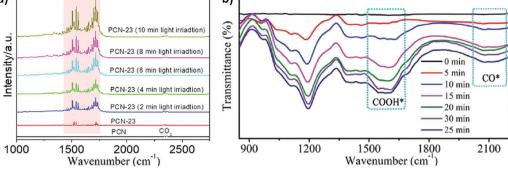
Fig. 11 In situ DRIFTS spectra illustrating the photocatalyzed CO<sub>2</sub> adsorption-activation over the surface of (a) PCN and defect rich PCN-23 (reproduced and modified with permission.<sup>42</sup> Copyright 2021, Elsevier) and (b) 3DOM CdSQD/NC (reproduced and modified with permission.<sup>20</sup> Copyright 2021, Wiley-VCH).
