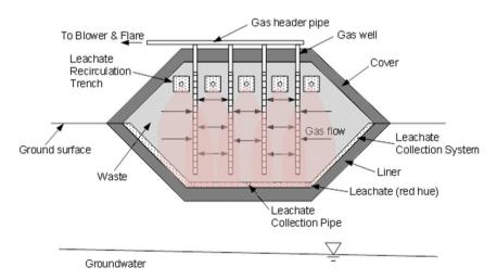
Fig. 9 MSW landfill with liner, cover, leachate collection, leachate recirculation, and gas collection.
