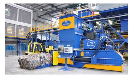
Fig. 11 Two-ram Baler from Machinex Recycling. Reproduced from ref. 104 with permission from Machinex Technologies, copyright 2022.
