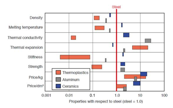
Fig. 5 Properties of thermoplastics, aluminum, and ceramics with respect to steel. Reproduced with permission from ref. 32 from Carl Hanser Verlag, Munich, copyright 2012.
