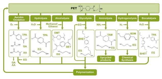
Fig. 28 Strategies for PET chemical recycling discussed in this section, and their most common products. (TPA = terephthalic acid, EG = ethylene glycol, DMT = dimethylterephthalate, DET = diethylterephthalate, BHET = bis-2-hydroxyethylterephthalate, BDM = benzenedimethanol, MHET = mono-2-hydroxyethylterephthalate.).
