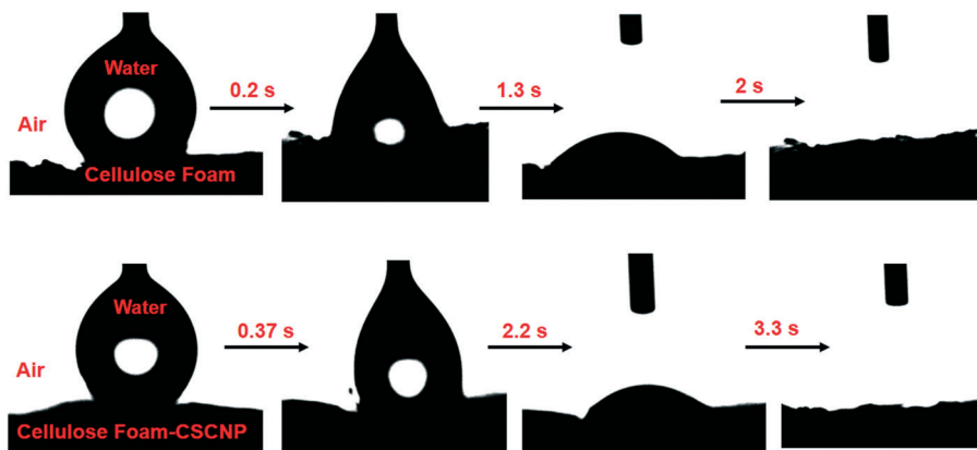
Fig. 5 Water contact angle measurements reveal the hydrophilic nature of the CF and CF-CSCNP surfaces, and indicate the water soaking behaviors with respect to time, captured through different image frames using a contact angle meter.
