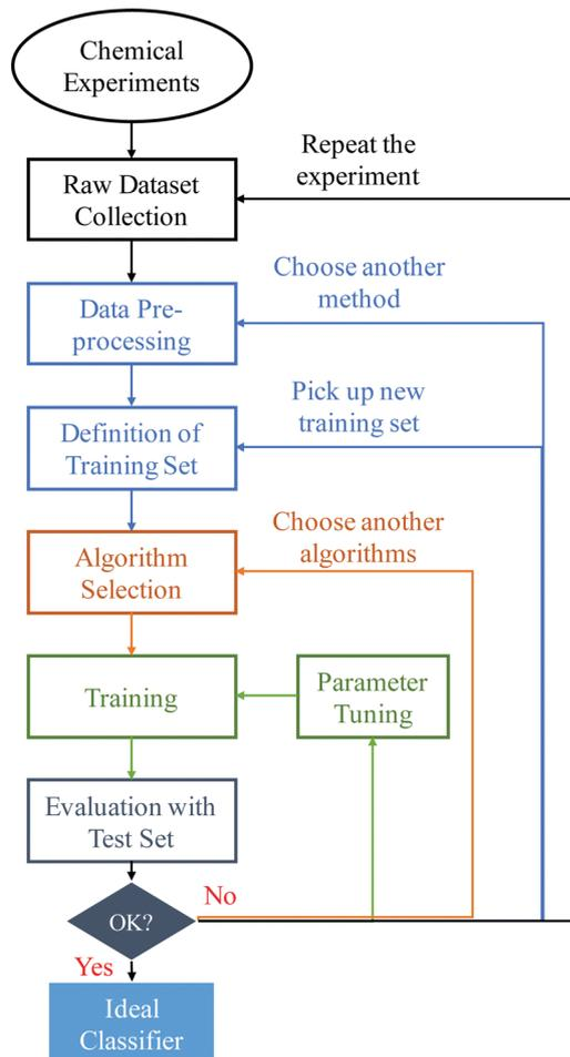
Fig. 25 Working flowchart of a supervised classification model to a chemical problem. The first step is to collect raw data from chemical experiments, and clean the dataset with various pre-processing methods. The second step is to select appropriate algorithms and initialize the classifier model. Then, split the dataset using cross-validation and feed the classifier model with the training data. Next, predict the label for test dataset, and evaluate the error rate of the classifier model.
