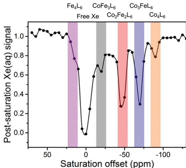
Fig. 11 CEST spectrum reported by Dmochowski and co-workers of a mixture of  $[\text{Xe} \subset \text{Co}_n\text{Fe}_{4-n}\text{L}_6]^{4+}$  host-guest complexes detected using hyperCEST. Adapted with permission from ref. 64. Copyright 2020 American Chemical Society.
