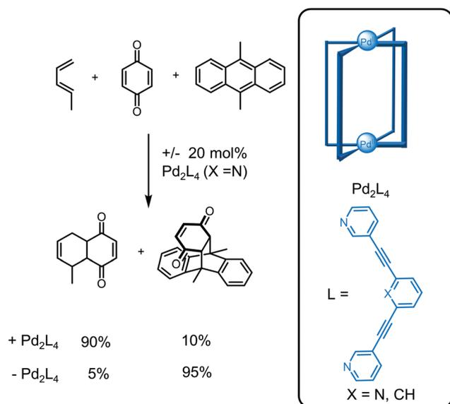
Fig. 17 Catalysis of Diels–Alder reactions by a  $Pd_2L_4$  cage (when  $X = N$ ) reported by Lusby and co-workers where the chemoselectivity is reversed in comparison to the uncatalysed reaction in the absence of the cage.
