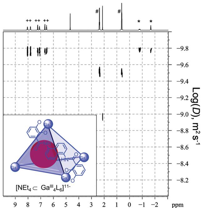
Fig. 10  $^1\text{H}$  and DOSY spectra of Raymond's  $[\text{NET}_4 \subset \text{Ga}^{\text{III}}_4\text{L}_6]^{11-}$  host-guest complex where the encapsulated  $\text{NET}_4^+$  guest is in slow exchange with "free"  $\text{NET}_4^+$ . Signals marked with + correspond to the cage, \* the encapsulated  $\text{NET}_4^+$  guest and # the "free"  $\text{NET}_4^+$ . Adapted with permission from ref. 62. Copyright 2008 American Chemical Society.
