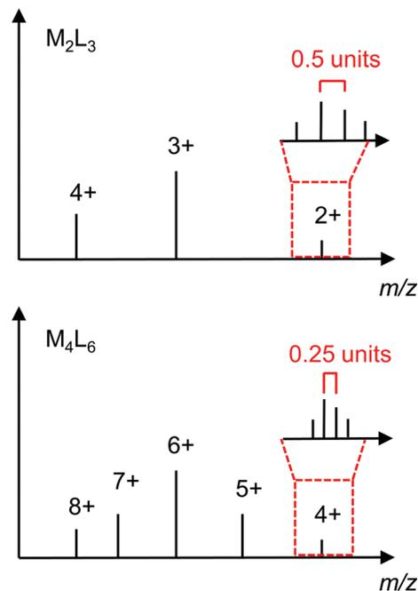
Fig. 12 Idealised mass spectra of  $\text{M}_2\text{L}_3$  and  $\text{M}_4\text{L}_6$  structures showing how they can be differentiated on the basis of the series of ion peaks and isotope pattern for a particular  $m/z$  ratio.
