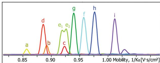
Fig. 13 Mobilogram of a mixture of 10 heteroleptic cages (a–i) reported by Clever and co-workers depicting the differentiation of the cages on the basis of their collision cross section (increasing from left to right) by trapped ion mobility mass spectrometry. Reproduced from ref. 71 with permission from the Royal Society of Chemistry.
