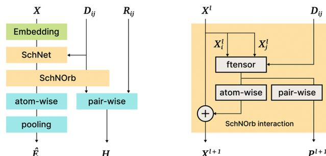
Fig. 6 The *SchNorb* architecture. On the left: general architecture overview; on the right: the *Interaction* block in *SchNorb*. In addition to the *SchNet Interaction* block, *SchNorb* uses the factorized tensor layer<sup>74</sup> to produce pairwise atom features and predict the basis coefficients for the Hamiltonian.
