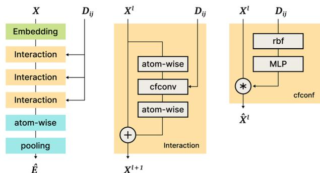
Fig. 3 A schematic depiction of the *SchNet* architecture with its sub-units. The left column shows an overview, and middle and right columns detail the Interaction and *cfconv* blocks.  $X$  is an atom's representation,  $D_{ij}$  is the pairwise distance matrix. Atom-wise blocks are multilayer perceptrons applied to each atom representation independently.
