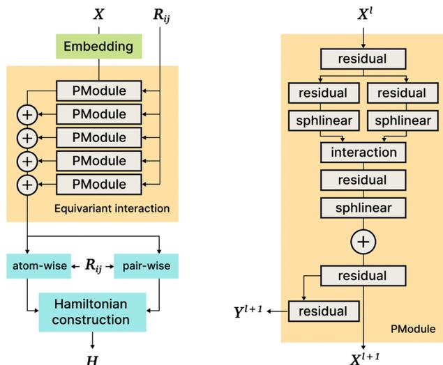
Fig. 7 *PhiSNet* architecture. On the left: General architecture overview; on the right: the *PModule* block in detail. More details about sphilinear and interaction blocks of *PModule* are given in phisnet2021.
