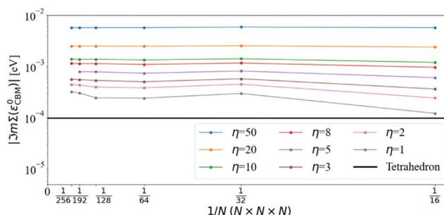
**Fig. 4** Convergence of  $\Im m\Sigma_{\text{CBM}}(\epsilon_{\text{CBM}}^0)$  using the DM approach with  $N$ , for different values of  $\eta$ , at 300 K. Exactly at the CBM, the standard method converges slowly down to the tetrahedron value, as the value of  $\Sigma$  is very small and comparable to the “infinitesimal”  $\eta$  itself. The tetrahedron value is calculated with  $N = 160$ . The y-axis is in logarithmic scale.
