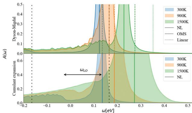
**Fig. 11** Spectral function calculated at the VBM at 300, 900, 1500 (K) using DM and CE methods. The vertical colored lines show the QP energy calculated using non-linear (NL), on-the-mass-shell (OMS) and linear approaches. The vertical dashed black lines correspond to  $\pm\omega_{LO}$ .  $\eta$  is set to 5 meV and  $N = 128$ .
