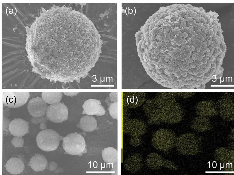
**Fig. 5** (a) High-magnification SEM images of ZIF-8/HSMC-SB<sub>Hmim</sub> and (b) ZIF-8/HSMC-SB<sub>Zn</sub>, (c) low-magnification SEM image, and (d) EDS mapping of Zn for ZIF-8/HSMC-SB<sub>Zn</sub>.
