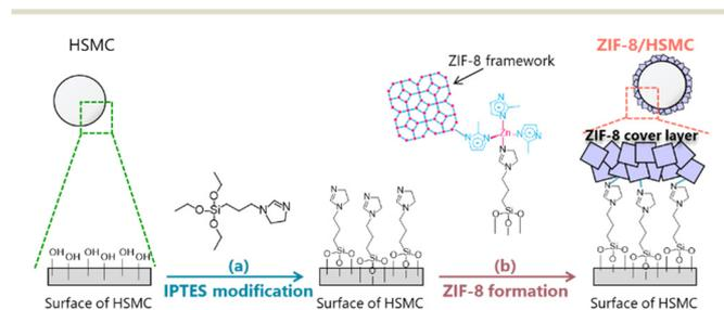
**Scheme 1** Schematic of the fabrication process for ZIF-8/HSMC. (a) IPTES modification process on the HSMC surface and (b) formation process for ZIF-8 cover layer using a batch operation or semi-batch operation.
