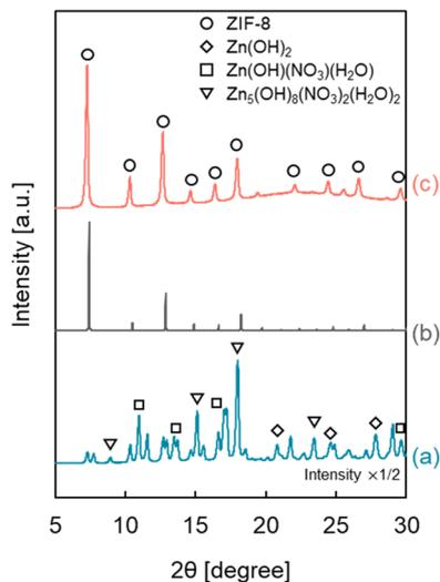
**Fig. 4** XRD patterns of the ZIF-8/HSMC-SB prepared by the semi-batch operation. (a) ZIF-8/HSMC-SB<sub>Hmim</sub> prepared by feeding the Hmim aqueous solution into the Zn<sup>2+</sup> aqueous solution, (b) simulated ZIF-8, and (c) ZIF-8/HSMC-SB<sub>Zn</sub> prepared by supplying the Zn<sup>2+</sup> aqueous solution into the Hmim aqueous solution.
