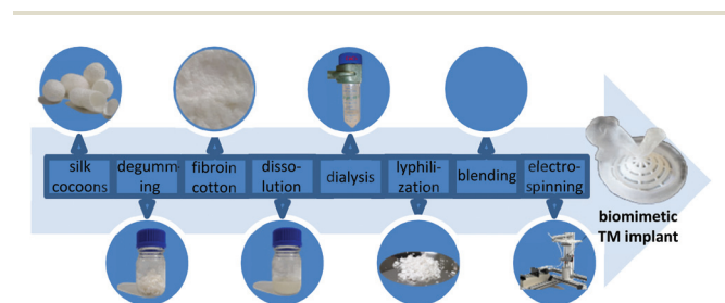
Fig. 1 Schematic workflow from Bombyx mori silkworm cocoon to a TM implant with morphologically biomimetic, mechanical and oscillatory properties.
