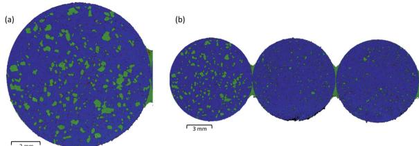
Fig. 3 LDIR chemical images of (a) a full single tablet and (b) three full tablets of the 3-component model system, where blue = microcrystalline cellulose, green = saccharin and red = hydrobromide salt API.
