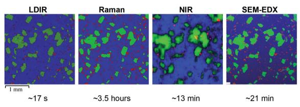
Fig. 2 (Left) LDIR, (left centre) Raman, (right centre) NIR and (right) SEM-EDX chemical images of the 3-component model system, where blue = microcrystalline cellulose, green = saccharin and red = hydrobromide salt API. Each chemical image represents a 3000  $\mu$ m  $\times$  3000  $\mu$ m area of sample and the total data collection time for each technique is displayed below the respective chemical image.
