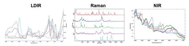
Fig. 4 The LDIR (left), Raman (centre) and NIR (right) spectra of the raw materials in the pharmaceutical tablet formulation where red = hydrobromide salt API, blue = microcrystalline cellulose, green = lactose monohydrate, magenta = croscarmellose sodium and cyan = magnesium stearate.
