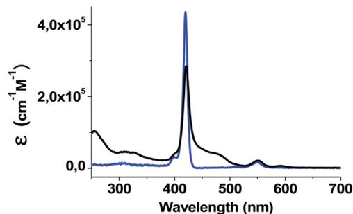
Fig. 4 UV-visible absorption spectra of ZnP-2EDOTV-C<sub>60</sub> (**1**, black) and ZnP (blue) in dichloromethane solution. Concentration: 10<sup>-5</sup> M.
