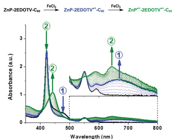
Fig. 5 UV-Vis absorption spectra of neutral (black), cation (blue) and dication (green) species of ZnP-2EDOTV-C<sub>60</sub> (**1**), in dichloromethane solution, generated upon successive additions of FeCl<sub>3</sub>.
