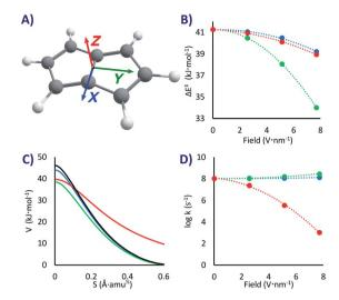
Fig. 2 (A) PL and the colour coded directing axes at which the EEF was applied. (B)  $\Delta E^{\ddagger}$  as a function of the field strength. (C) Potential energies at the M06-2x/6-311G(d) level vs. the reaction mass-scaled coordinates (only one side of the symmetrical PES is shown); in black the profile without EEF, blue, green and red are with 7.7 V nm<sup>-1</sup> fields in the X, Y, Z directions, respectively. (D) Tunnelling rate constants from the ground state vs. the field strength.
