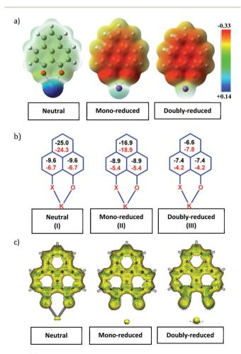
Fig. 2 (a)Total charge density plots of the three redox states of the PLY(O,O)–K complex (Isovalue 0.002); (b) NICS values for **1a** (in black) and **1b** (in red) of the three different redox states; (c) anisotropy of the Induced Current Density (ACID) plots of **1a** in the three different redox states.
