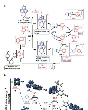
Fig. 4 (a) Proposed mechanistic cycle for the C–H arylation reaction by aryl halide activation; (b) reaction pathway by DFT calculations along with the geometry and spin density plot ( $\alpha$ -spin in blue and  $\beta$ -spin in green color) of the reactive intermediates and transition states.
