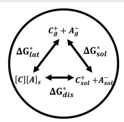
Fig. 2 Schematic representation of the thermodynamic cycle for dissolution of [cation][VBH] complexes. The free-energy of dissolution  $(\Delta G_{\mathrm{dis}}^*)$  determines the solubility of the complex and results from the interplay between the free-energy of the lattice  $(\Delta G_{\mathrm{lat}}^*)$  and that of stabilizing solute–solvent interactions in solution  $(\Delta G_{\mathrm{sol}}^*)$ .
