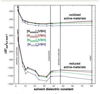
Fig. 8 DFT-calculated values of  $\Delta G_{\mathrm{sol}}^*$  for reduced and oxidized  $[N_{XXXX}]_{\nu}[VBH]$  compounds in various solvents with dielectric constant varying between 2 and 80 (X = 1 to 4, and Y = 2 for reduced species and Y = 1 for oxidized species)
