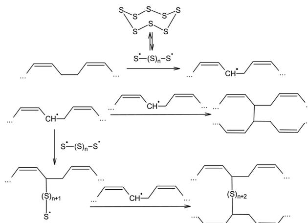
Scheme 2 Mechanism of the vulcanisation of *cis*-poly(buta-1,3-diene).
