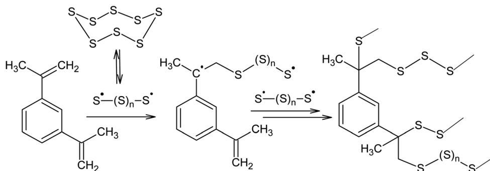
Scheme 3 Reaction between S<sub>8</sub> and 1,3-diisopropenylbenzene.
