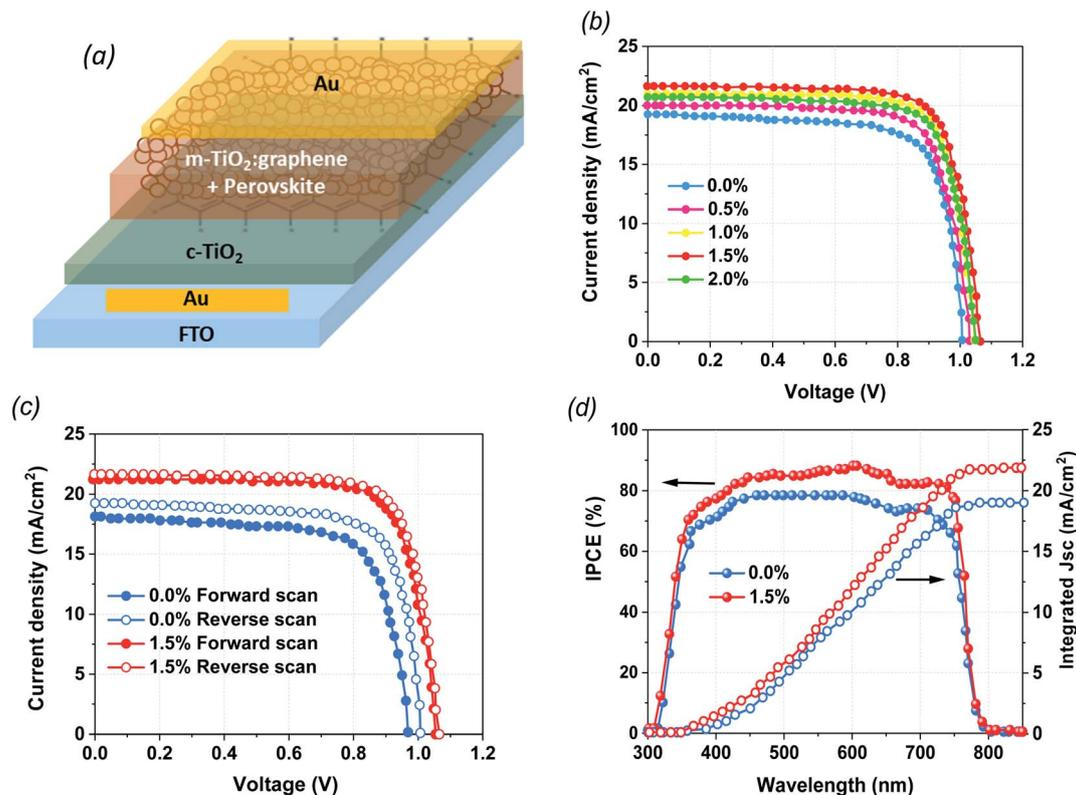
Fig. 1 (a) Schematic illustration of the architecture of the devices fabricated in this study. (b)  $J$ - $V$  plots of PSCs with different amounts of graphene (0.0%, 0.5%, 1.0%, 1.5%, and 2.0%) in the G/TiO<sub>2</sub> layer. (c) Hysteresis effect of PSCs with pure TiO<sub>2</sub> and TiO<sub>2</sub> containing 1.5% graphene. (d) EQE spectra of PSCs with and without graphene doping.
