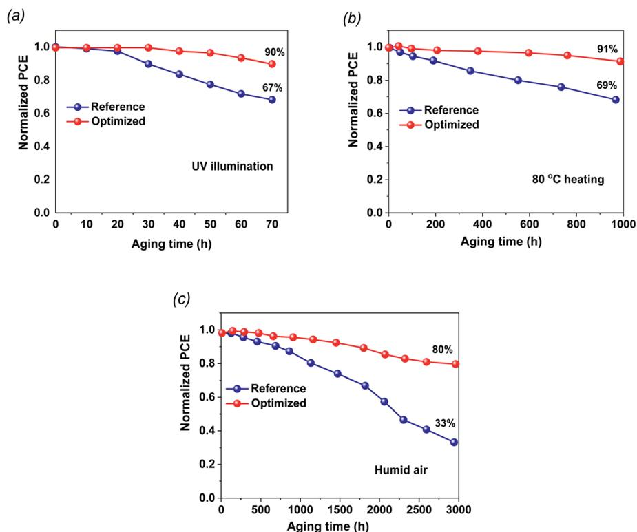
Fig. 5 Stability performance of PSCs under various conditions. All the devices are unencapsulated and the reference devices are compared with 1.5% graphene-containing devices. (a) Stability test of the perovskite device on  $\text{TiO}_2$  and on G: $\text{TiO}_2$  ETLs under continuous UV light illumination at room temperature. (b) Devices kept at 80 °C under a nitrogen atmosphere. (c) Devices in ambient air with a RH of 25–35% at room temperature.
