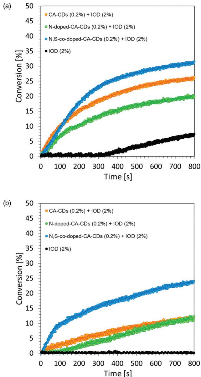
**Fig. 10** Free-radical photopolymerization profiles (acrylate function conversion vs. irradiation time) for TMPTA with the bimolecular photoinitiating system based on IOD (2.0 wt%) and CDs (0.2 wt%) (a) under irradiation at 365 nm; (b) under irradiation at 405 nm. Irradiance was measured at a distance of 210 mm for all sources.
