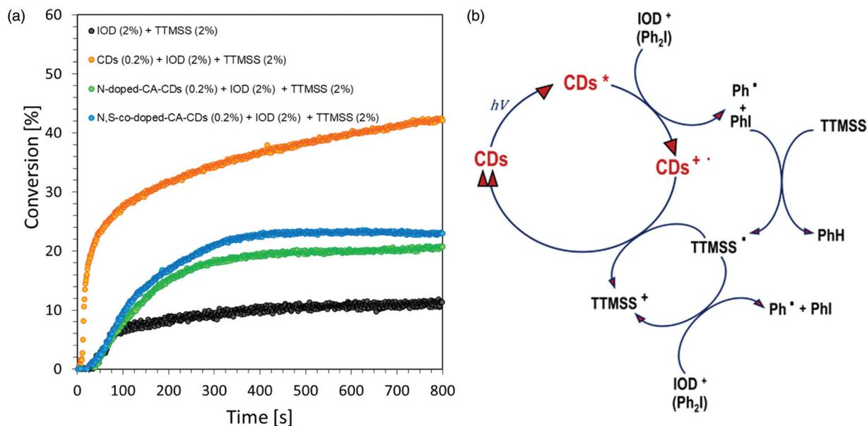
**Fig. 9** (a) Cationic photopolymerization profiles (epoxy function conversion vs. irradiation time) initiated by a photoinitiating system based on IOD (2.0 wt%), TTMS (2.0 wt%) and CDs (0.2 wt%) under irradiation at 405 nm. (b) Schematic cycle of operation of the initiating system consisting of IOD, TTMS and CDs.
