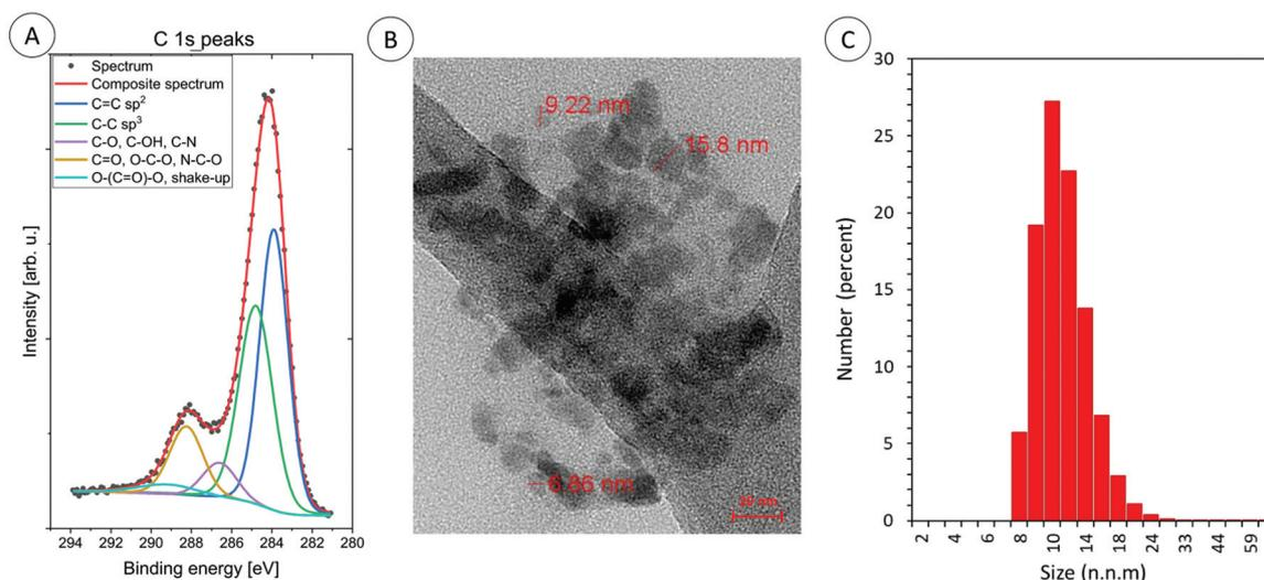
Fig. 4 (A) The high energy resolution XPS spectra of C 1s peaks for carbon dots: CA-CDs, (B) TEM image of carbon dots: CA-CDs, and (C) DLS particle size distribution histogram of CA-CDs.
