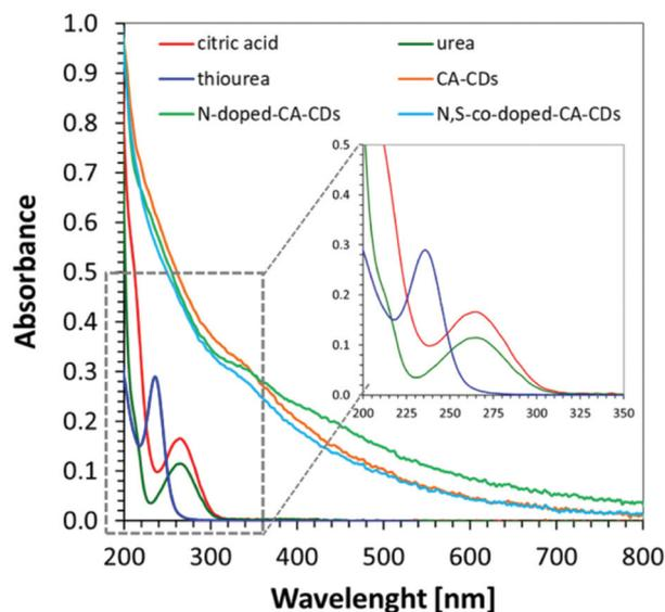
Fig. 5 UV-visible absorption spectra of the synthesized citric acid-based CDs (CA-CDs, N-doped-CA-CDs, N,S-co-doped-CA-CDs) dissolved in water ( $0.01 \text{ g mL}^{-1}$ ) and the organic molecular precursors for the synthesis of CA-CDs.
