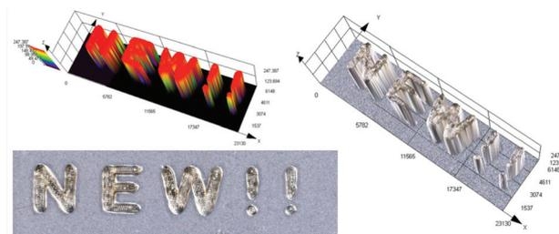
**Fig. 14** 3D hydrogel inscription made by the free-radical photopolymerization of a HEA/water (1/1 wt%) mixture in the presence of a two-component photoinitiating system based on CA-CDs (0.2 wt%) and IOD (2 wt%).
