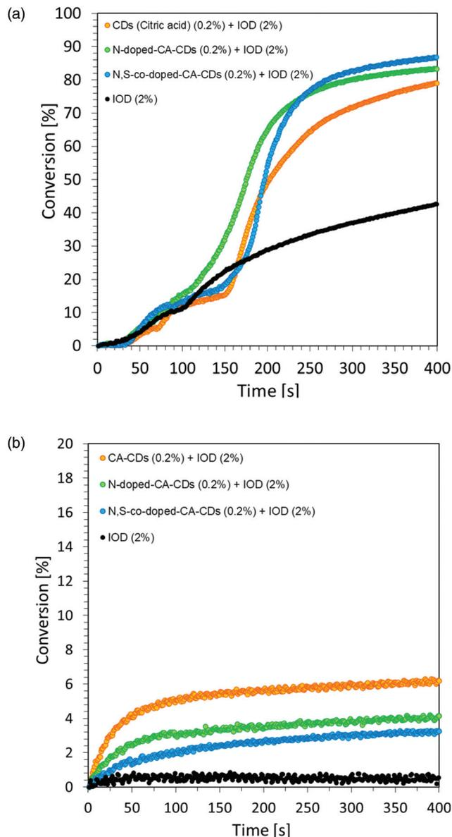
**Fig. 7** Cationic photopolymerization profiles (vinyl function conversion vs. irradiation time) initiated by a bimolecular photoinitiating system based on IOD (2.0 wt%) and CDs (0.2 wt%) (a) under irradiation at 365 nm and (b) under irradiation at 405 nm.
