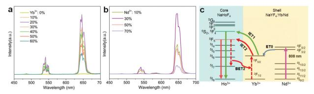
Fig. 5 (a and b) Upconversion emission spectra of NaHoF<sub>4</sub>@NaYF<sub>4</sub>:Yb(0-60 mol%) and NaHoF<sub>4</sub>@NaYF<sub>4</sub>:Yb (20 mol%)/Nd (10-70 mol%) core-shell nanoparticles under 980 and 808 nm excitations, respectively. (c) Schematic of the energy transport processes in the Nd<sup>3+</sup>-sensitized upconversion system.
