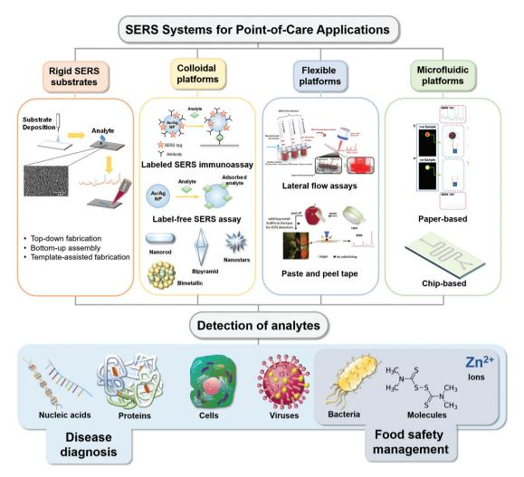
Scheme 1 Schematic illustration of reported various types of point-of-care SERS platforms and the different types of analytes detected for various applications. Reproduced with permission from ref. 51. Copyright 2019, Elsevier. Reproduced with permission from ref. 98. Copyright 2020, Royal Society of Chemistry. Reproduced with permission from ref. 139. Copyright 2017; Elsevier.
