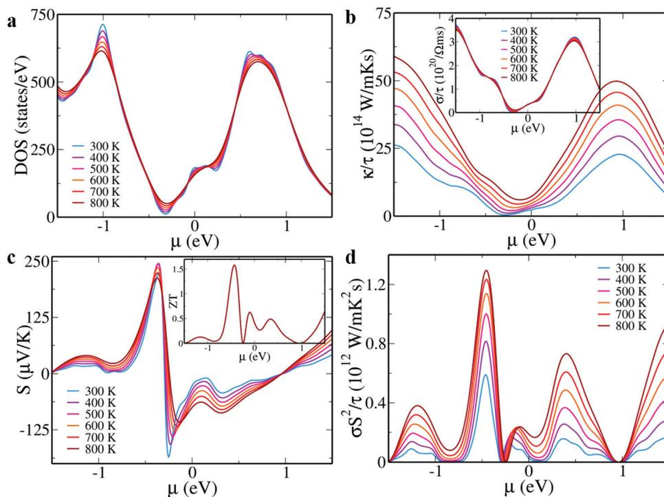
Fig. 3 (a) DOS; (b) thermal conductivity (inset: electrical conductivity); (c) Seebeck co-efficient (inset:  $ZT@800\text{ K}$ ) and (d) power factor of  $\text{Sn}_{10}\text{Pb}_5\text{BiTe}_{16}$  as a function of chemical potential ( $\mu$ ) at various temperatures. The conductivity and power factor values are reported by scaling it with  $\tau$ .
