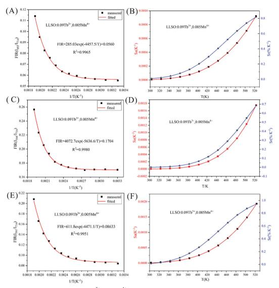
Fig. 8 FIR values,  $S_r$  and  $S_a$  values of La<sub>2</sub>LiSbO<sub>6</sub>:0.09Tb<sup>3+</sup>,0.005Mn<sup>4+</sup> at different temperatures.
