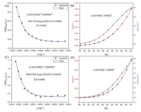
FIR values,  $S_r$  and  $S_a$  values of La<sub>2</sub>LiSbO<sub>6</sub>:0.09Dy<sup>3+</sup>,0.005Mn<sup>4+</sup> at different temperatures.
