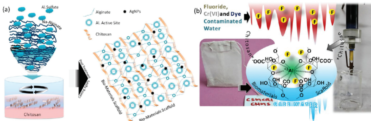
Fig. 10 (a) Schematic representation of the preparation of an aluminium-composite-impregnated sodium alginate and chitosan-based biomaterial scaffold. (b) Shows the application of the bio-composite for the separation of dyes, Cr(VI) and fluoride through a teabag model and a continuous flow method. 277
