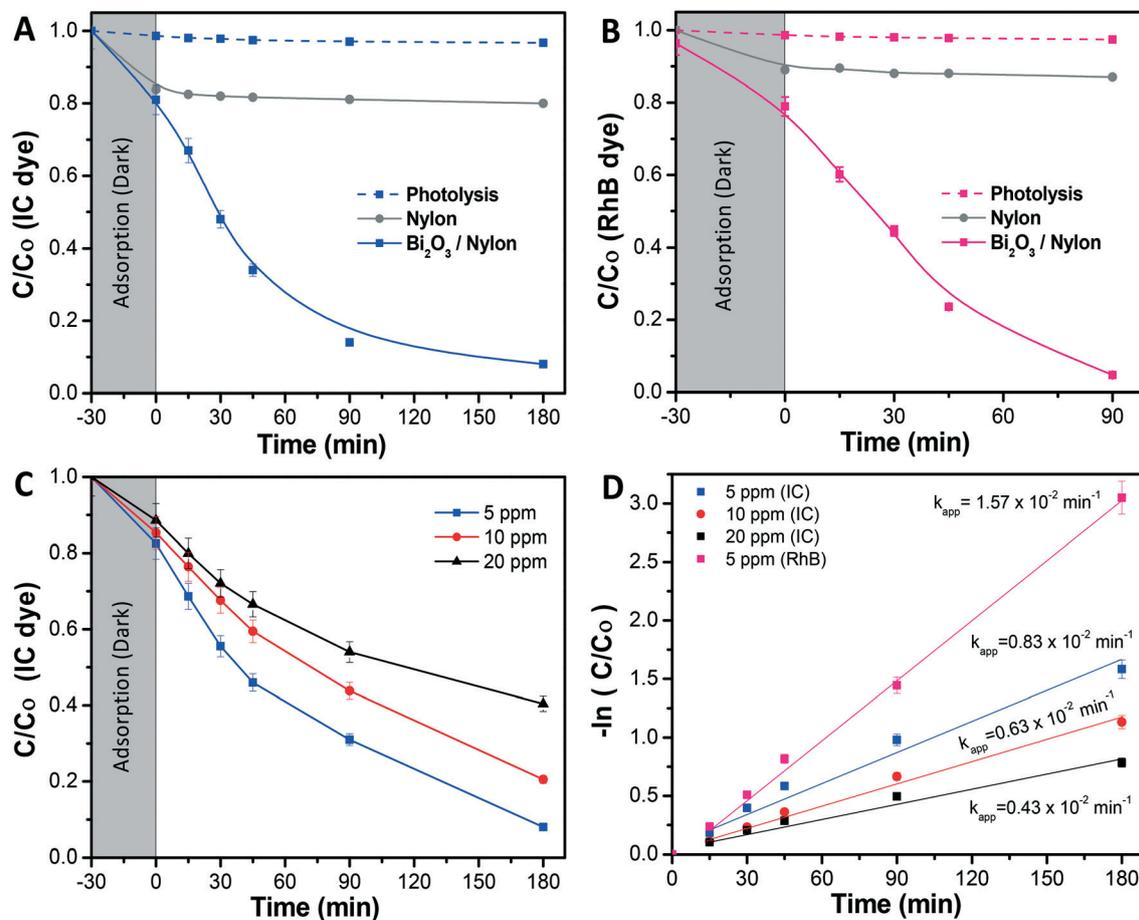
Fig. 6 Photocatalytic tests using bare nylon and  $\text{Bi}_2\text{O}_3/\text{nylon}$  composite membranes: A) relative concentration ( $C/C_0$ ) of IC degradation vs. time ( $C_0 = 5\text{ ppm}$ ); B)  $C/C_0$  of RhB degradation vs. time ( $C_0 = 5\text{ ppm}$ ); C)  $C/C_0$  of different IC dye concentrations with the  $\text{Bi}_2\text{O}_3/\text{nylon}$  composite membrane; and D) kinetic curve of IC and RhB dye solutions, and estimated apparent kinetic rates ( $k_{app}$ ).
