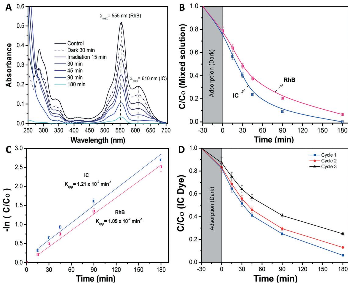
**Fig. 7** A) Absorbance spectra vs. irradiation time of the mixed solution, B) relative concentration ( $C/C_0$ ) of combined dyes degraded using the  $\text{Bi}_2\text{O}_3/\text{nylon}$  composite, C) kinetic curves of removal of IC and RhB dyes in the mixed solution, and estimated  $K_{\text{app}}$ , and D) cyclic stability of the  $\text{Bi}_2\text{O}_3/\text{nylon}$  composite membrane up to three cycles;  $C/C_0$  profiles at 5 ppm IC dye concentration.
