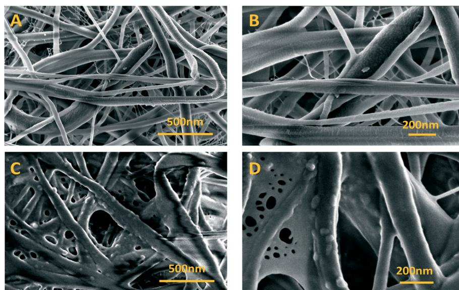
Fig. 3 FESEM images of bare nylon and Bi<sub>2</sub>O<sub>3</sub>/nylon membranes at different magnifications. (A) Bare nylon (25k×), (B) (50k×), (C) Bi<sub>2</sub>O<sub>3</sub>/nylon (25k×), and (D) (50k×).
