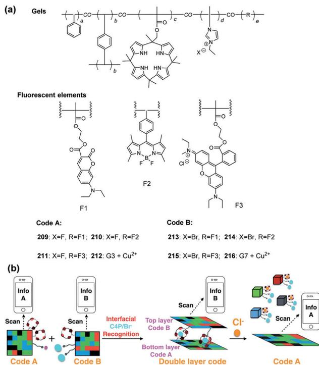
Fig. 32 (a) Chemical structures of the polymeric gels, the incorporated fluorescent elements, and the recognition elements present in Code A (**209–212**) and Code B (**213–216**). (b) The mechanism of forming a double layer code and specific sensing of Cl<sup>-</sup> anions.
