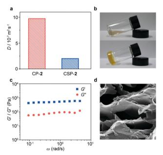
Fig. 3 (a) Diffusion coefficient D (500 MHz,  $CD_3CN/CDCl_3 = 3:1 \text{ v/v}$ , 298 K) of CP-2 and CSP-2. (b) Images of CP-2 solution (above) and CSP-2 gel (below). Solvent: CH<sub>3</sub>CN: CHCl<sub>3</sub> = 3:1 v/v, 2.0 mL. (c) Storage modulus G' and loss modulus G'' versus frequency ( $\omega$ ) for the CSP-2 gel. (d) The SEM image of the freeze-dried CSP-2.
