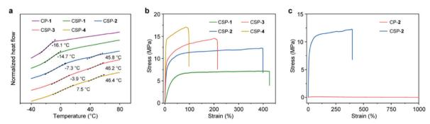
Fig. 4 (a) DSC curves of CP-1 and CSPs-1-4 recorded by heating scan from -40 to 80 °C with a heating rate of 20 °C min<sup>-1</sup>. (b) Tensile stress-strain curves of CSPs-1-4 in the bulk. Deformation rate: 20 mm min<sup>-1</sup>. (c) Tensile stress-strain curves of CP-2 and CSP-2 samples in the bulk. Deformation rate: 20 mm min<sup>-1</sup>.
