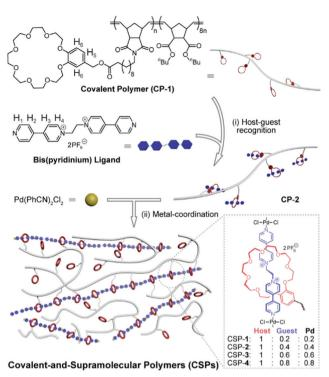
Fig. 1 Schematic representation of the formation of synergistic CSPs and chemical structures of the CP-1 and bis(pyridinium) ligand.
