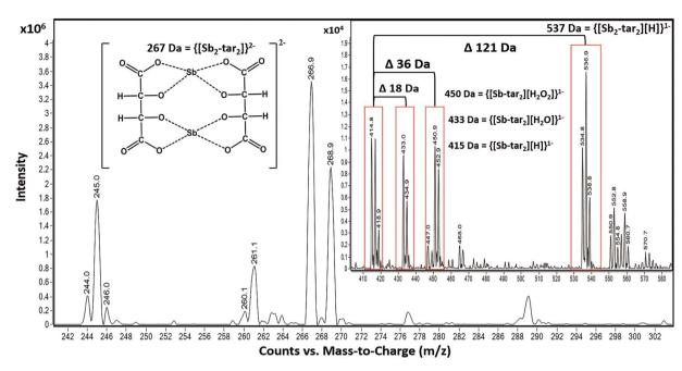
Fig. 4 Flow injection analysis of the various tartrate complexes with Sb in ESI- mode. Adducts formation is still prevalent, and because of the nature of the ligand, multiple Sb ions can bind to multiple ligands. For instance, the difference between 415 Da and 433 Da is an m/z value of 18, a water molecule. However, from 415 Da to 537 Da is the addition of an Sb ion.
