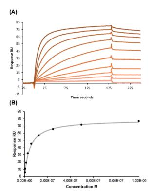
Fig. 4 SPR analysis of interaction between Fuc-Ub and immobilized BambL. (A) Sensorgram of multiple cycle affinity analysis consisting of injections of increasing concentration (1 nM to 1  $\mu$ M) of Fuc-Ub. (B) Affinity analysis based on data from (A).
