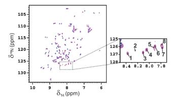
Fig. 5  $\,^{2}$ D  $^{1}$ H $^{-15}$ N HSQC spectra of WT-Ub (blue) and WT-Ub functionalized with the fucosyl derivative 7 on the Lys sidechains (Fuc-Ub, magenta) acquired at 298 K and 700 MHz. The signals in the area, selected by the dashed lines (enlarged on the right), correspond to the new amide groups obtained by the conjugation of the  $\epsilon$ -NH $_{2}$  group of lysine sidechains and the N-terminus with fucoside 7.
