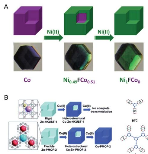
Fig. 8 (A) Synthetic scheme for the preparation of core-shell heterostructures *via* selective transmetalations. Reproduced with permission from ref. 78. Copyright 2012, American Chemical Society. (B) Transmetalations in two MOFs (Zn-HKUST-1 and Zn-PMOF-2) with different framework flexibilities. Reproduced with permission from ref. 108. Copyright 2012, Royal Society of Chemistry.
