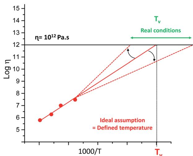
Fig. 9 Example of imperfect evaluation of the topology freezing temperature ( $T_v$ ) caused by measurement errors, based on standard deviations and small temperature window or unconsidered low temperature interactions.
