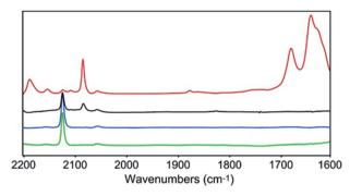
Fig. 4 IR-SEC of complex 1 in dry CH<sub>3</sub>CN with 0.1 M TBAPF<sub>6</sub> at resting potential under Ar (green), CO<sub>2</sub> (blue), and at -2.24(11) V vs. Fc/Fc<sup>+</sup> under Ar (black) and CO<sub>2</sub> (red). LabOMak IR-SEC cell equipped with Pt grid for working and counter electrodes and CE and Ag pseudoreference electrode.
