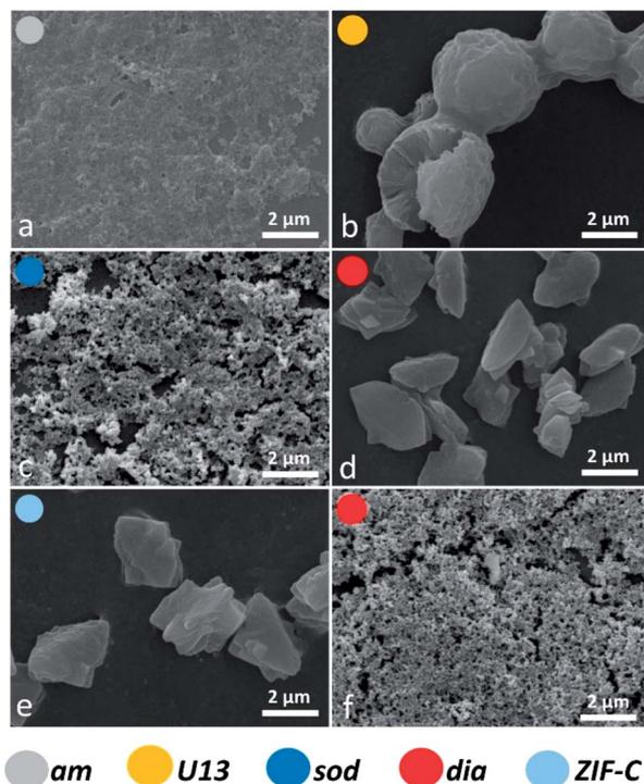
Fig. 4 SEM micrographs of the biocomposites *am* (a) and *U13* (b, from TD-H<sub>2</sub>O), *sod* (c, from TD-EtOH), *dia* (from TD-H<sub>2</sub>O) (d) and from TD-EtOH (f) and *ZIF-C* (e, from TD-H<sub>2</sub>O) phases. *ZIF-C* refers to ZIF-CO<sub>3</sub>-1.<sup>40</sup>
