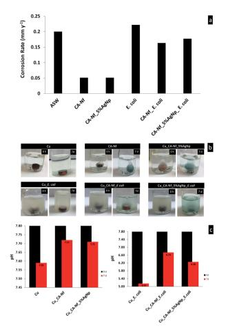
Fig. 7 Cu, Cu coated CA-Nf and Cu coated CA-Nf with 5% AgNps in the ASW and ASW inoculated with  $E.\ coli$  (a) corrosion rates values (mm  $y^{-1}$ ) (b) photographs of the Cu discs weight loss analysis and (c) pH changes.
